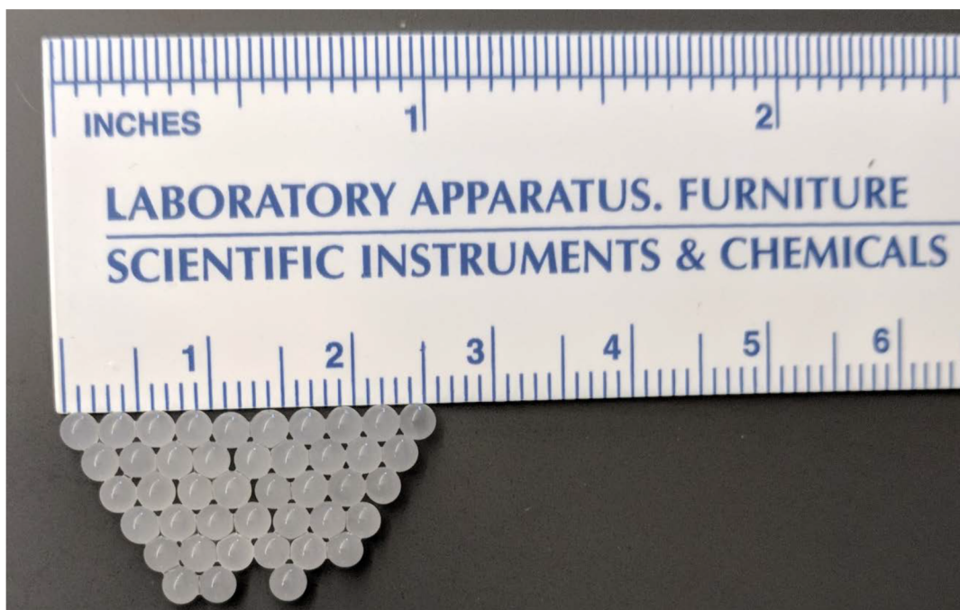
Figure S 7.2. Gelated alginate macrobeads with a VWR ruler for scale.
