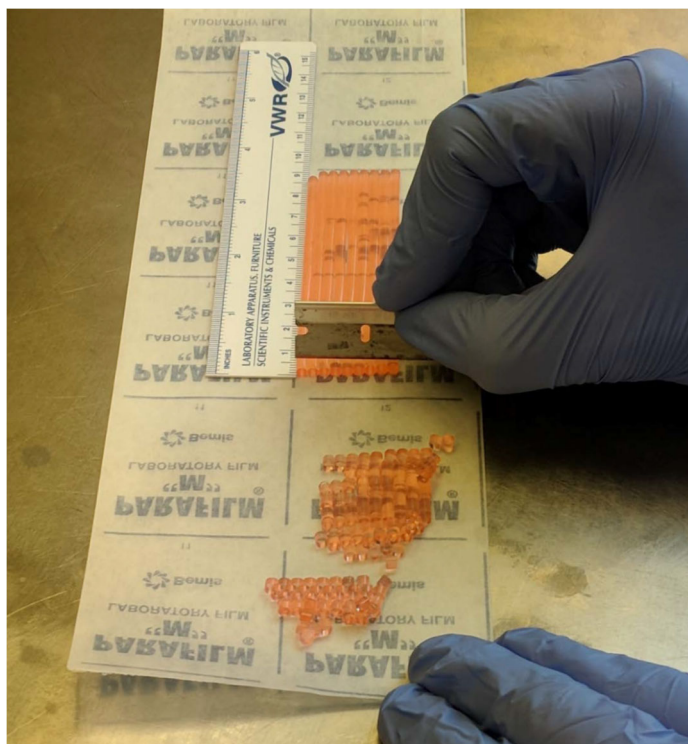
Figure S 7.5. Manual cutting of gellan-gum strands into 2mm right cylinders for experimental use. For better visualization GG pre-gel solution was dyed orange.
