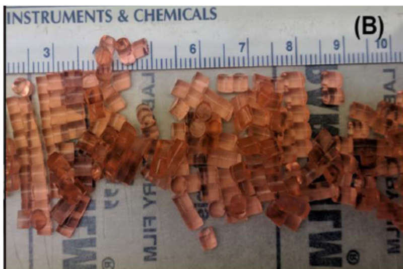
Figure S 7.6. Gellan-gum beads with R. rhodochrous ATCC 21198 and TBOS co-encapsulated 2 mm in diameter by 2 to 3 mm in length.
