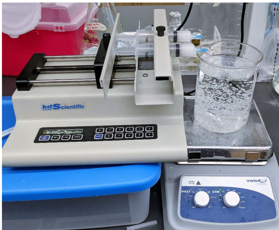
Figure S 7.1. Calcium-alginate macrobead formation by extrusion into crosslinking solution.
