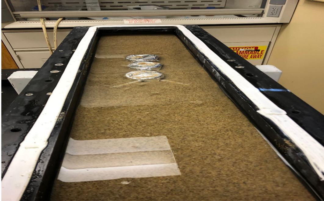
Figure 9.3. The PAM packed with accusand sand 20-30 mesh and three bioreactors which can be packed gellan-gum macrobeads co-encapsulated with R. rhodochrous ATCC 21198 and TBOS and T2BOS.
