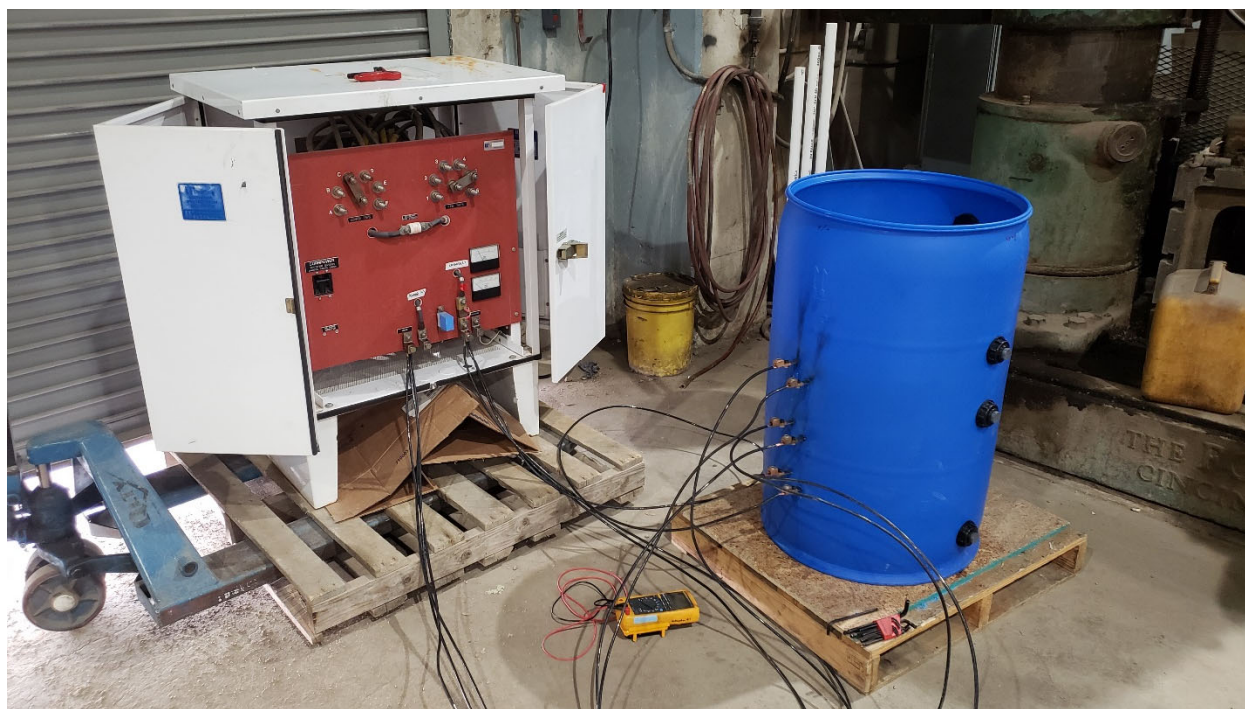
Figure 40: Drum-scale bioelectrochemical reactor and rectifier for field testing, designed and constructed at Colorado State University in collaboration with Jacobs.
