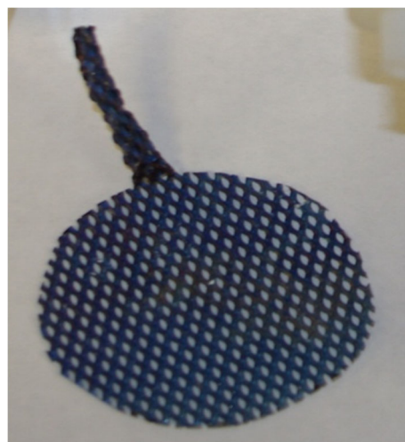
Figure 4: Ti-MMO mesh electrode processed for flow-through column installation.
