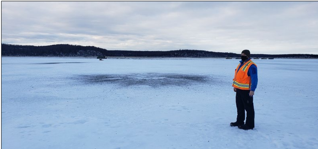
Figure 4. Depositional plume from live fire of a study cartridge with IMP fuze setting.
