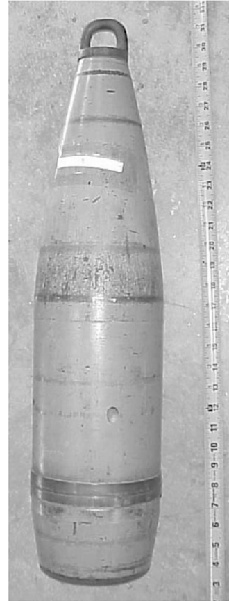
This 155mm artillery round is similar to the one detected below ground at Aberdeen Proving Ground MD.
