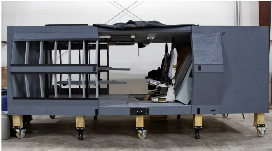
Figure 1. Wooden MEDEVAC simulator.
