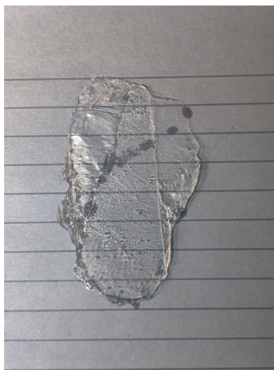
Figure 3.3: Gel polymer electrolyte hand pressed for lab-scale prototypes.
