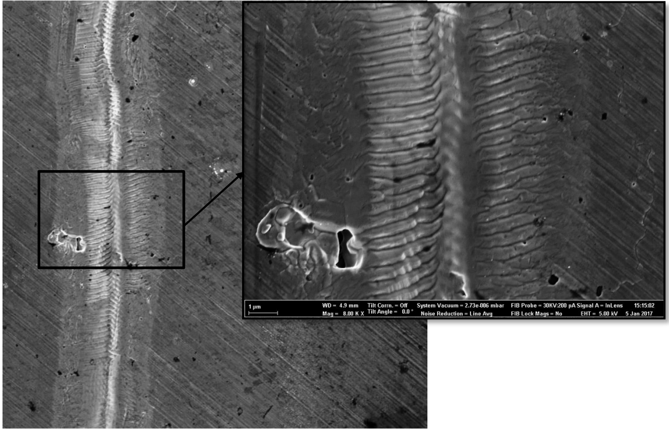
Figure 82. SEM image of line 0.01 mm/s in vacuum.
