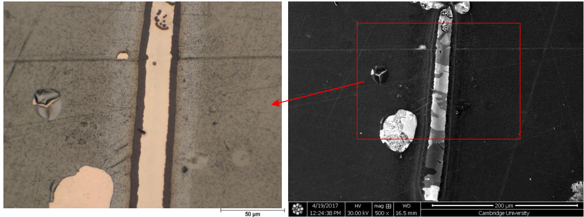
Figure 76. OFHC Cu coated with 100 nm Ti, treated with 50.5 kJ/cm 2 a) optical and b) FIB images.
