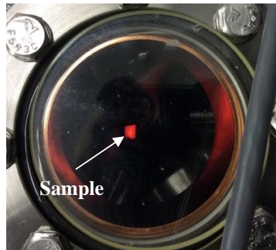
Figure 36. Image of the 316 SS sample through the window of the AMCS chamber, 19.17 \text{ kJ/cm}^2 , during e-beam bombardment with 50 keV.
