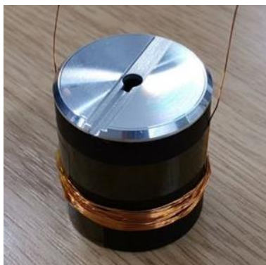
Figure 98: Tufnol test cup for a first test. After the cup is filled with LN, the aluminium lid with a sample is added. The whole in a lid is supposed to redirect the evaporated fumes to the back of the sample to cool it. The copper wire is an aid to lower the cup into a LN dewar avoiding unnecessary spillage.
