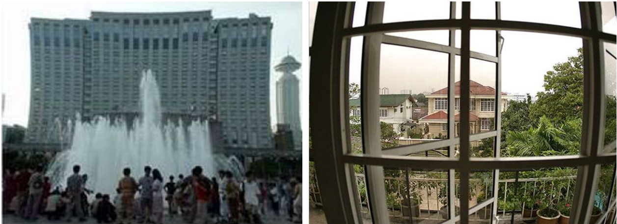
Figure 1 Pincushion (left) and barrel (right) distortion effects
