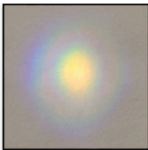
Figure 55. Photograph of the SC generated by 1318 nm on a white piece of paper.
