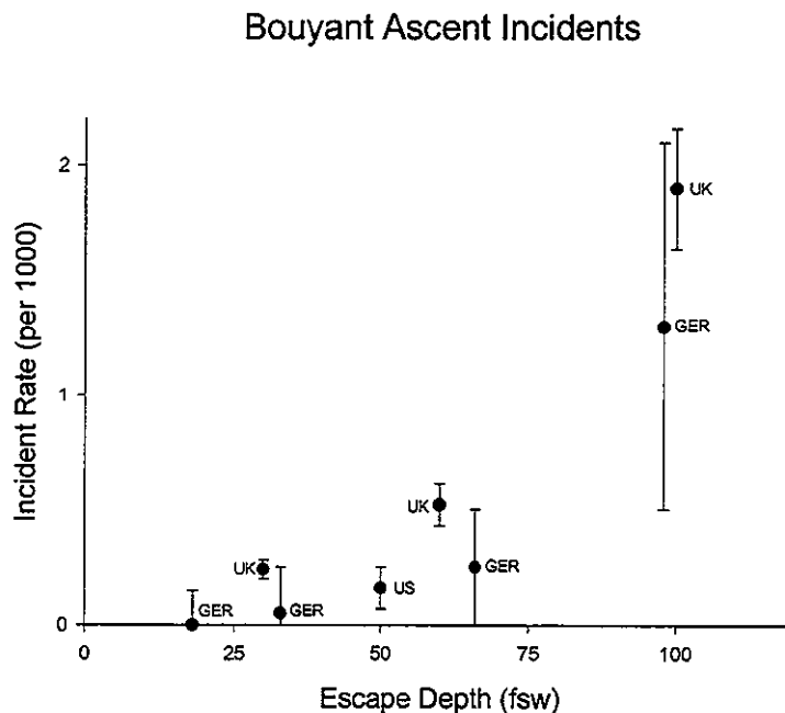
Figure 3. Graphical representation of various reported incident rates (+/- 1 SD) associated with depth from which submarine escape training is conducted. UK refers to reports from the Royal Navy, US refers to reports from the U.S. Navy, and GER refers to reports from the German Navy.
