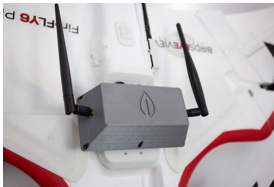
Figure 3. Data Mule Payload mounted on BirdsEyeView Firefly6 Pro airframe.
