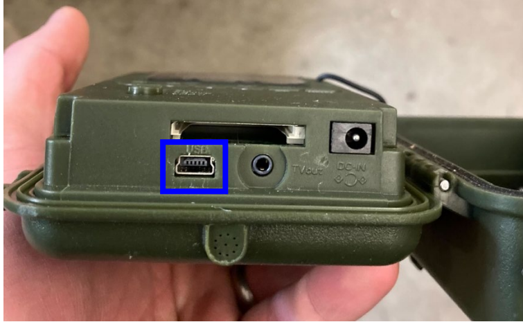
Figure 4. USB Mini port on the sensor (outlined in blue) is needed for out-of-the box compatibility with the Data Mule technology.
