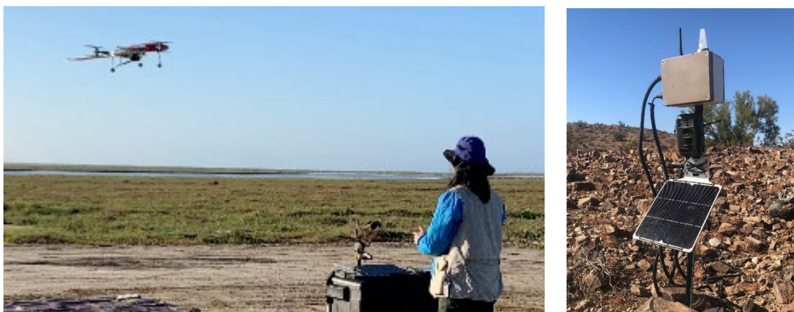
Figure 2. UAS with the attached payload supervised by an operator (left) and ground station, with communications box, camera trap, and solar panel (right).
