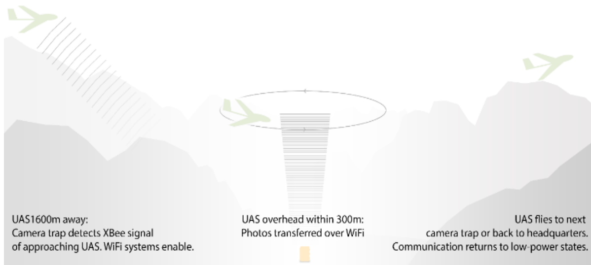
Figure 1. Overview of UAS Data Mule data download process.
