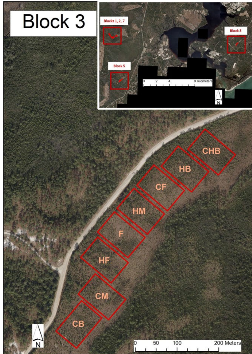
Figure 3. Layout of Block 3, with eight experimental units representing eight different site preparation treatments. Treatments are combinations of two vegetation control methods ('H' = herbicide; 'C' = chopping) and three soil manipulation methods ('B' = bedding; 'F' = flat-planting; 'M' = mounding).
