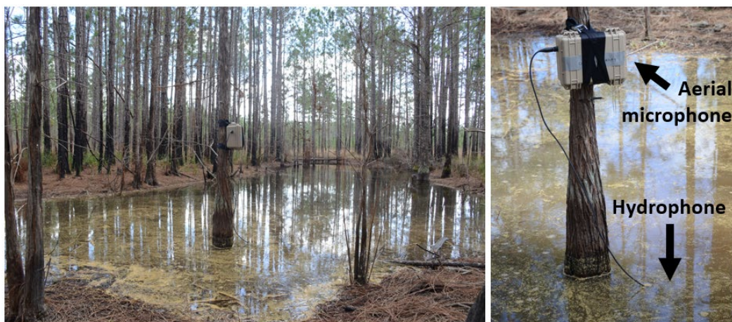
Figure 9. Swift recording unit equipped with microphone (PAM) and hydrophone (SPAM) at wetland D at Fort Stewart, GA, in 2018. This wetland was resampled in 2019 based on gopher frog detection in 2018.
