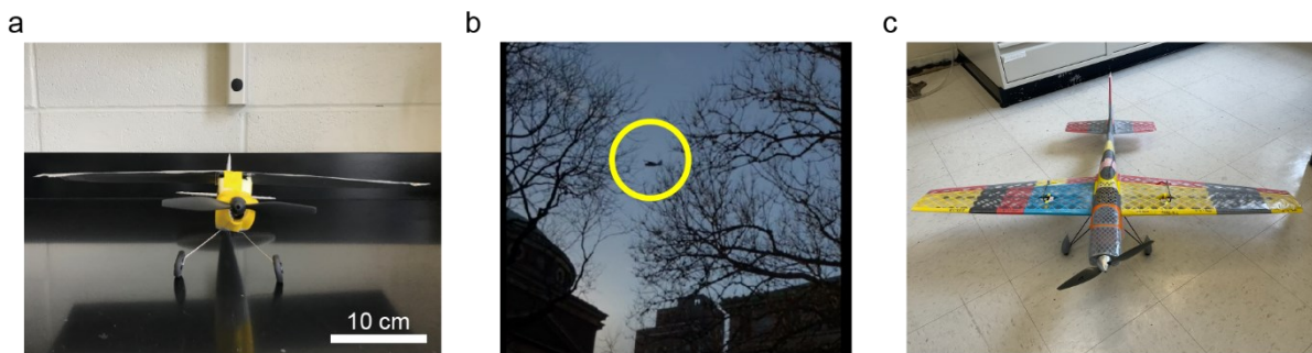
Figure 7. (a) Front view of a model airplane with laminated pouch cells as “electric wings”. The airplane is 44 cm \times 35 cm \times 12 cm (L \times W \times H), and it can fly steadily with the wing cells as the only power source. A single-layer electrode is 17.3 cm \times 7.5 cm (L \times W) in one wing, and one wing can provide a capacity of 780 mAh. (b) The model airplane was flying in the sky, which is in the yellow circle. (c) A 3D printed airplane model with a wingspan of \sim 1.5 m, which serves as a platform to test structural batteries. We plan to cover the wings with structural batteries in the next step.
