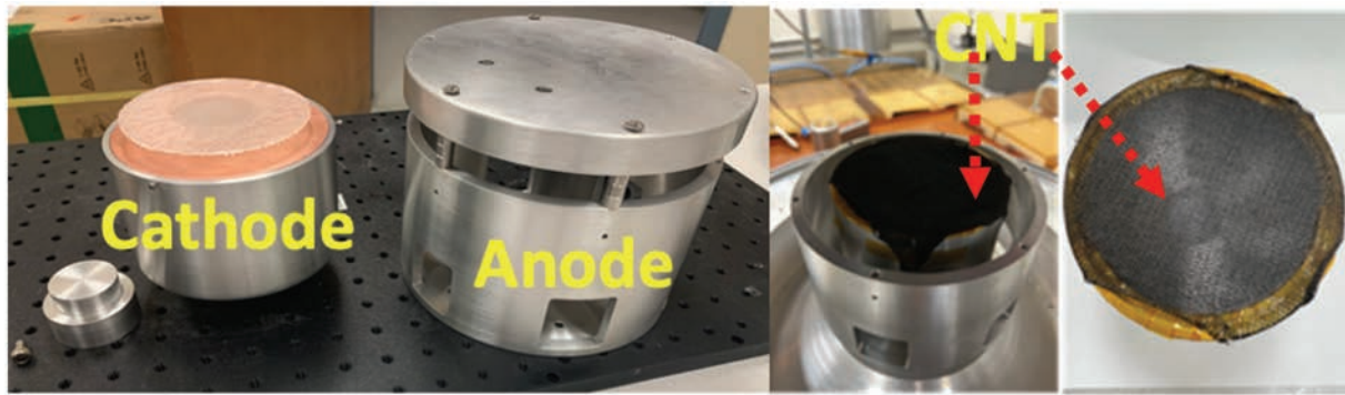
Figure 21. Typical hardware and assembly of a CNT cathode fired on the LOBO LTD. The left image shows the cathode holder next to the anode assembly. The latter can hold various anode materials although it was not possible to carry out the latter experiments with materials other than Al. The two far right images show the CNT cathode in place.
