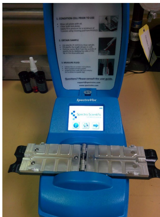
Figure 3. Sample Cell Micro-Channels of the SpectroVisc Q3050 Used for Viscosity Measurement
