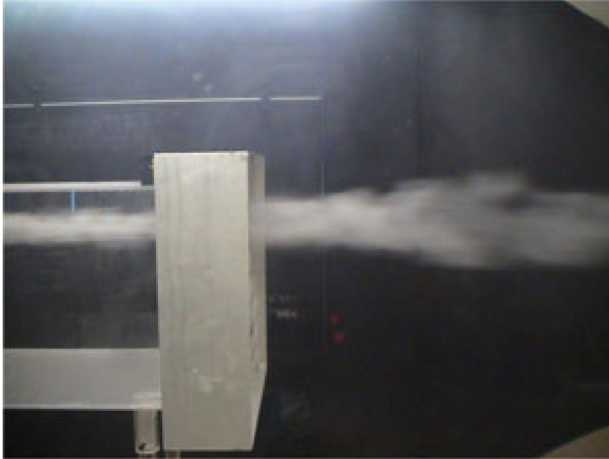
Figure 5. Smoke visualization of fractal grid turbulence.
