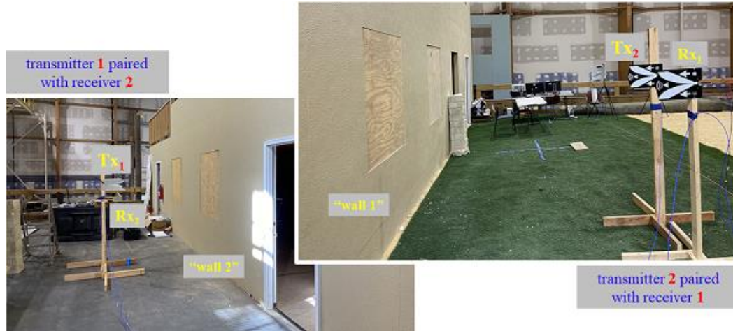
Fig. 25 Experiment at ARL-ALC Building 507: Tx antenna connections swapped to simulate a bistatic radar
