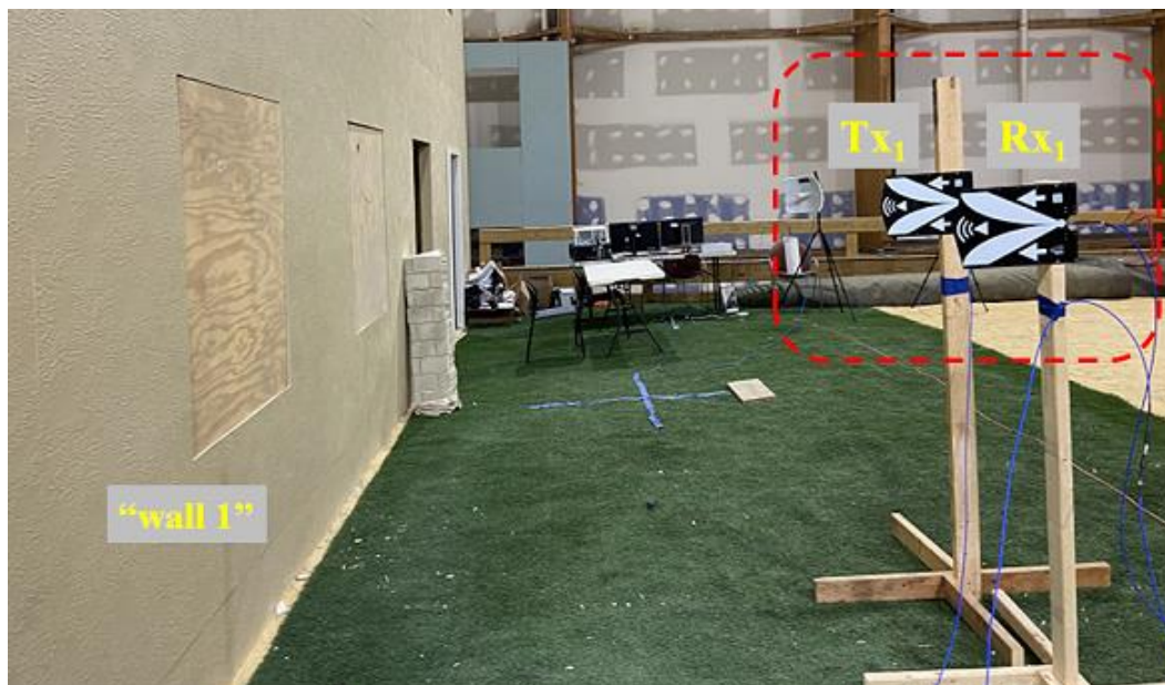
Fig. 3 Experiment at ARL-ALC Building 507: Tx_1 and Rx_1 antennas pointed at the plywood building outside of “wall 1”
