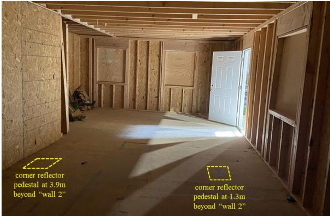
Fig. 15 Inside the plywood building: locations of corner reflectors toward/away from antenna pair Tx_2/Rx_2
