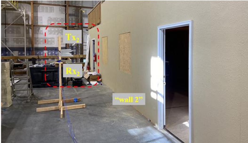
Fig. 4 Experiment at ARL-ALC Building 507: Tx_2 and Rx_2 antennas pointed at the plywood building outside of “wall 2” (door was closed during active data collections)
