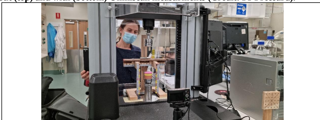
Figure 18. E8-114a experiments: Overview of the test rig including Instron machine used to perform with physical phantom of the replica tissues (skin, fat, muscle) of the residuum without (top) and with (bottom) Omniscan measurments (Credit: PI-Frossard).
