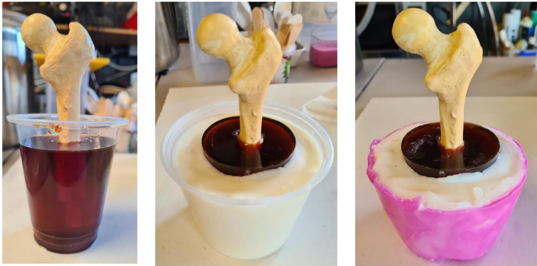
Figure 28. E9-E13 Experiments: Design of physical phantom including femur (Plastic), muscle (Gelatine), fat (Lard, pork fat), skin (Pinkysil silicone) (Credit: CI-Langton).
