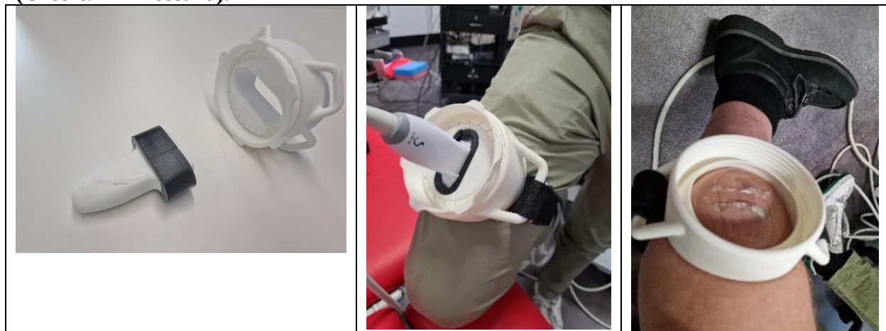
Figure 42. E17-E43 Experiments: Design and trial of 3D printed ultrasound probe holder (Credit: PI-Frossard).
