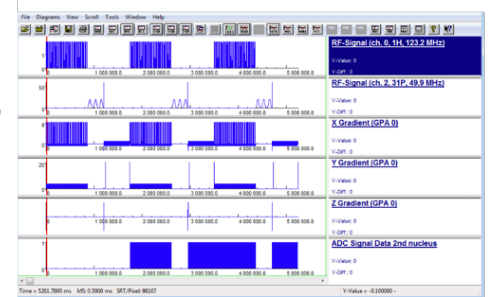
Fig. 1. A) Interleaved multinuclear ^1\text{H}/^{23}\text{Na} spectroscopic FID pulse sequence diagram in Siemens IDEA software. B) Resulting proton ( ^1\text{H} ) and B) sodium ( ^{23}\text{Na} ) FID including both real (top) and imaginary (bottom) quadrature channels. D) Interleaved, multinuclear gradient echo imaging (FLASH) pulse sequence diagram and E) this diagram implemented in Siemens IDEA software environment. F-G) Constructed saltwater phantom with different concentrations of sodium. H) Simultaneous sodium and I) proton FLASH images of the saltwater phantom. J) Interleaved single echo ^1\text{H} -CEST-EPI/ ^{23}\text{Na} -FLASH pulse sequence diagram and K) this diagram implemented in Siemens IDEA software environment to run on the 3T Prisma scanner.
