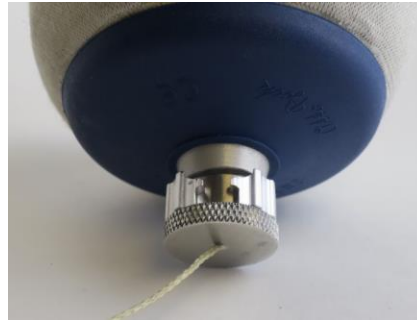
Fig. 4. Quick Pin final design. The user rotates the yellow knob, slides the pin into the slot, and then releases the yellow knob to lock the pin in place.
