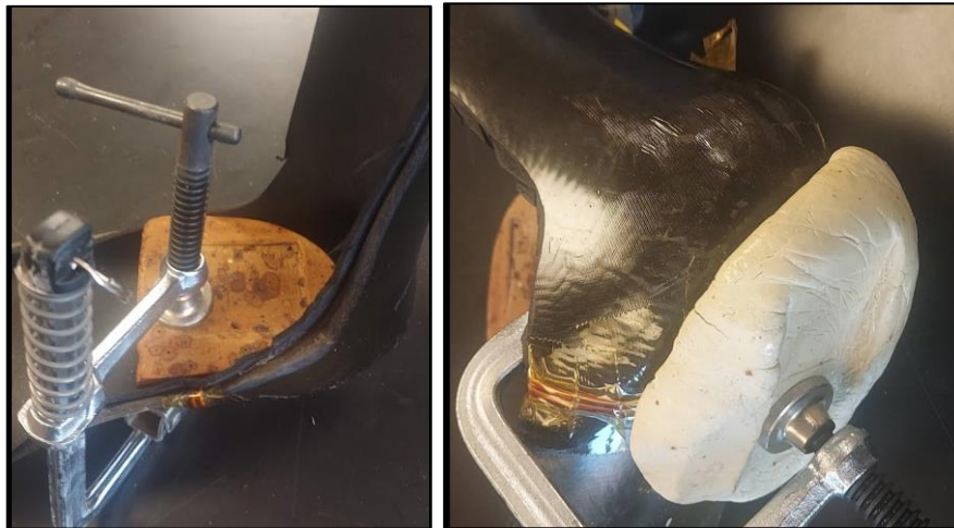
Fig. 28. Revised clamping procedure for holding the strain gages to the footplate during curing. Custom molds are fabricated, and a spring clamp is used.
