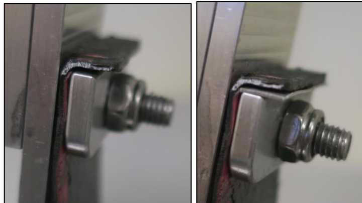
Fig. 38. Shims introduced at the ends of the carbon fiber strut. The shims are placed between the restraint plate and end of the strut.
