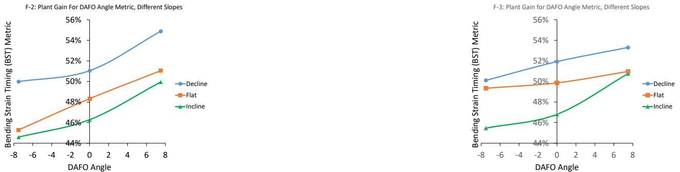
Fig. 17. Plant gain results for DAFO angle (in degrees) – surface terrain slope introduces a meaningful disturbance. Data for participants F-2 and F-3 are shown. Data were not available for participant F-1.
