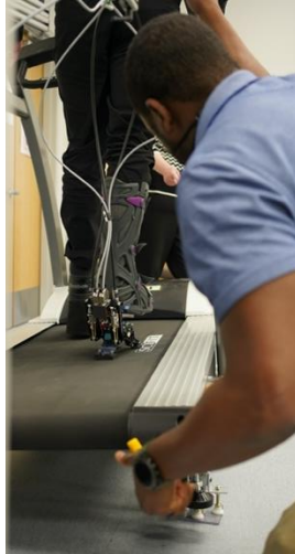
Figure 10. Research prosthetist adjusting the treadmill belt to prevent belt slippage when the treadmill is pitched at a cross sloped angle.
