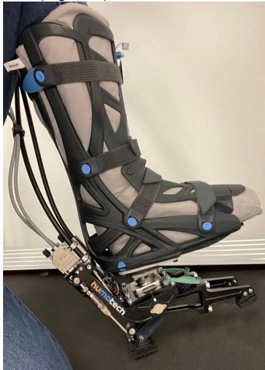
Figure 9. Multiaxial prosthetic foot emulator end effector shown connected to a simulator boot.
