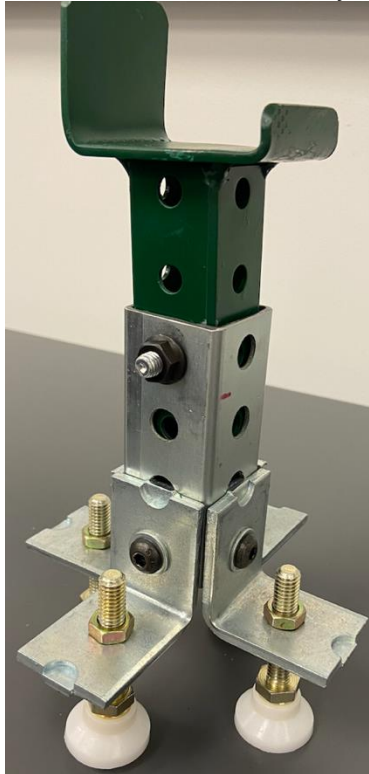
Figure 2. Custom jack that will be used to support the SciFit treadmill during cross-slope walking conditions for human subjects data collection.
