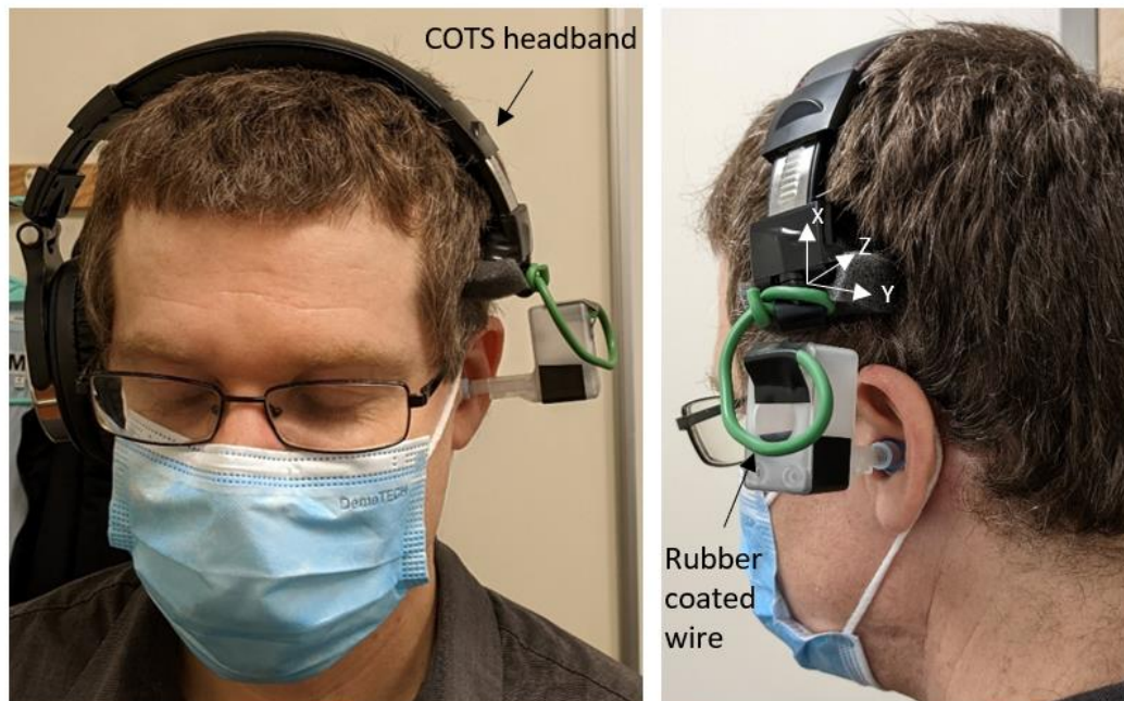
Figure 8. Our Next Generation Design Concept. This combines a COTS headband and adjustable wire to provide comfort to the patient and flexible placement to the audiologist.
