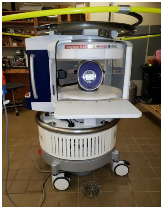
Figure 3. The portable, point-of-care 64 mT clinical MRI scanner (Hyperfine “Lucy”) in the Goodson Lab at SIUC. Scanner runs with a wireless (iPad), and DICOM images are stored on a cloud server.
