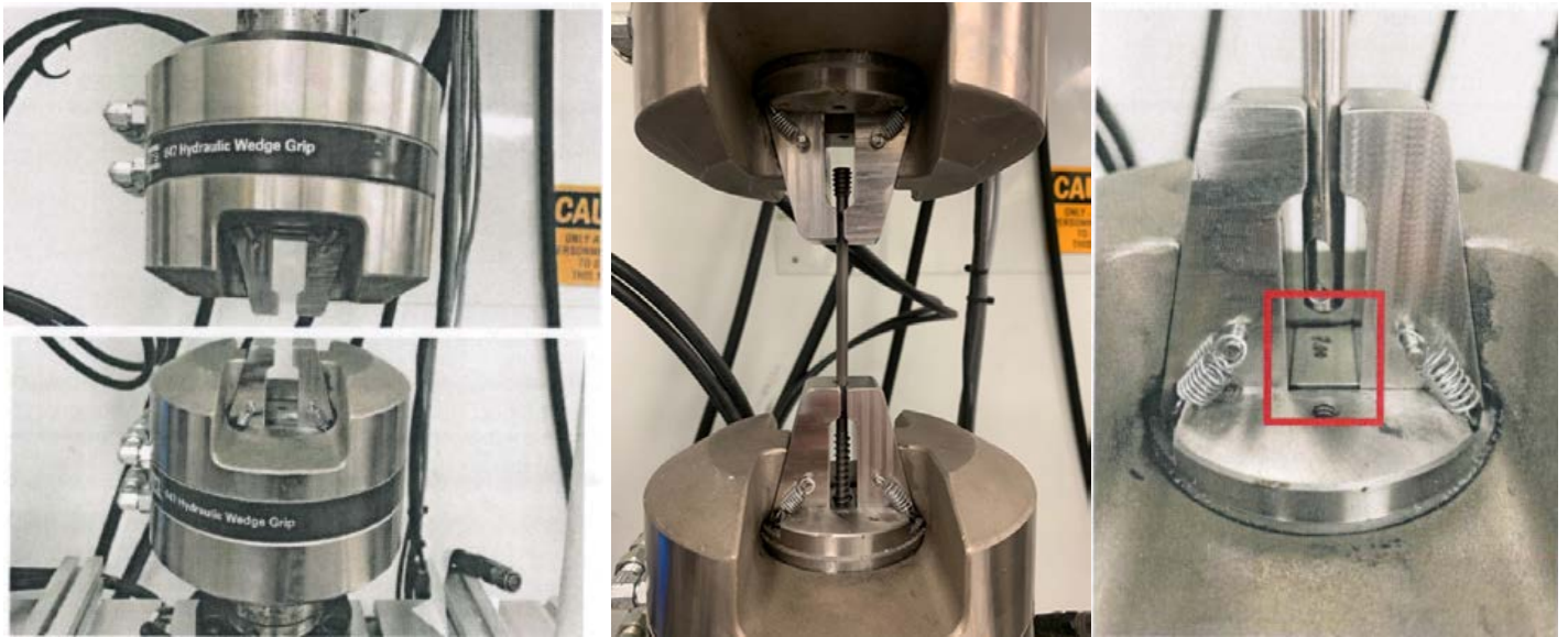
Figure 14. (left) Upper and lower pneumatic grips with custom torsion fixtures. (center) Inset view with predicate device clamped in fixture for torsion testing. (right) Inset view with prototype device clamped in fixture for torsion testing.
