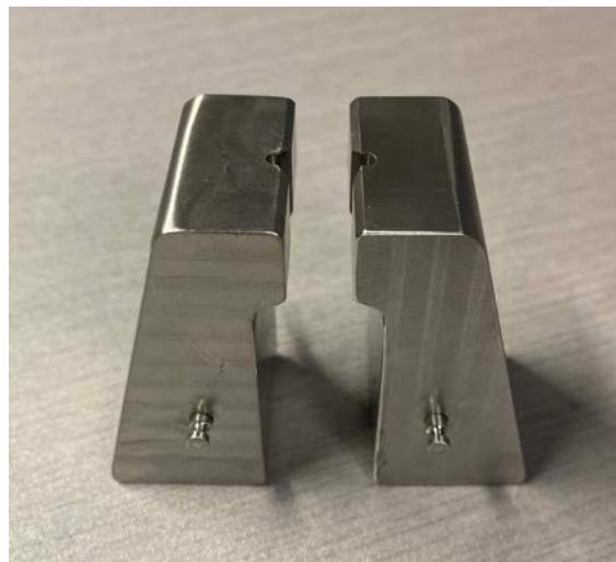
Figure 13. Machined set of grips for torsion testing.
