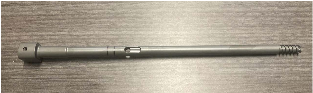
Figure 23. Fully assembled device with nail guide on left side and dynamic prototype device on right side.
