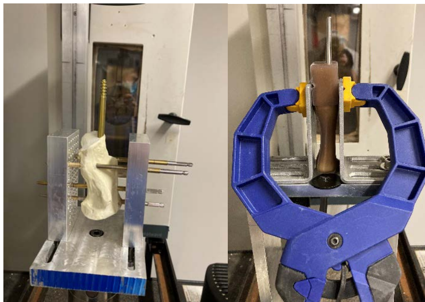
Figure 5. Test setup for determining pull-out force in (left) synthetic calcaneus and (right) synthetic metatarsal.
