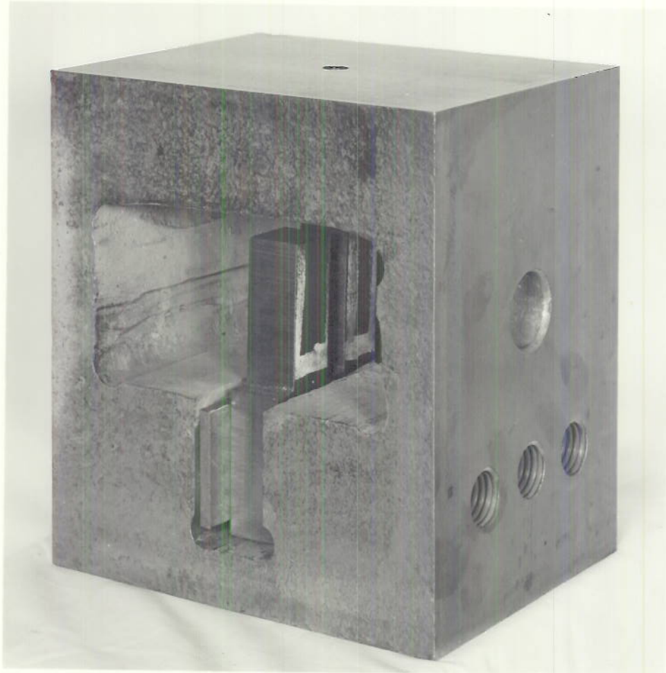
100 POUND JIG USED FOR HOLDING NRL SHOCK FRACTURE SPECIMENS
