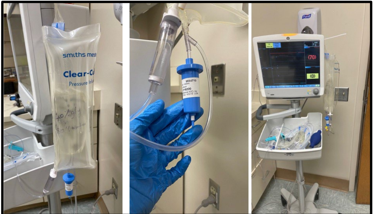
Figure 6. The bag filled with blood analog solution is pressurized to deliver the flow through the cortical vein model at a velocity of 1 cm/s. As the degree of stenosis is varied within each venous limb, the pressure before and after the one-way valve within the cortical vein is measured and displayed on the monitor in real-time.
