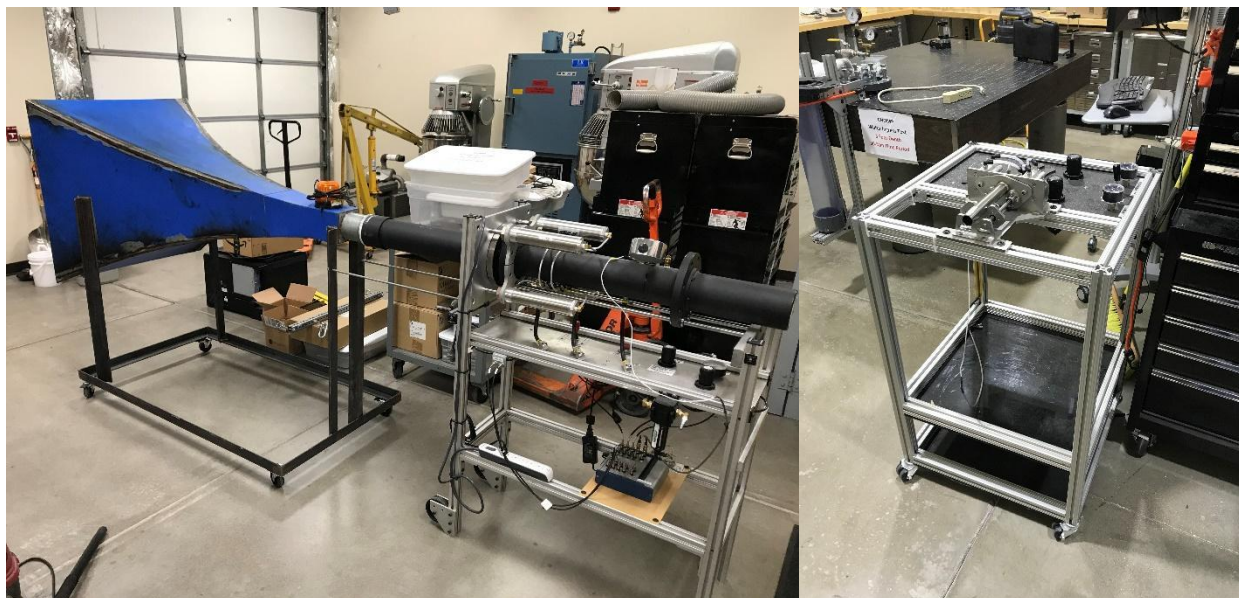
Figure 36. (Left) ARA ANSI-compliant shock tube and (Right) short duration shock tube for eIN testing.
