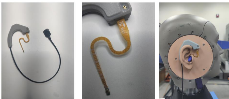
Figure 4. (Left) Completed prototype in-ear microphone assembly with flex circuit and preamp. (Center) Close-up on the in-ear flex circuit. (Right) The in-ear microphone assembly mounted on the 45CB test fixture and inserted alongside an HPD.
