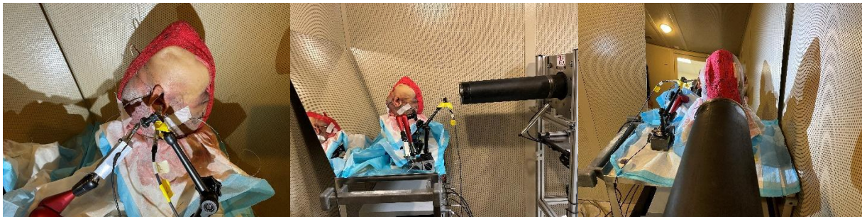
Figure 28. Equipment and specimen setup for PMHS shock wave exposures. The equipment and specimen were mounted on a mobile cart and elevated to center the specimen in front of the shock tube outlet. Pressure sensors were inserted into the cochlea and held in place using stainless steel guide tubes but were damaged during testing regardless. Greater efforts to protect the entire length of the sensor cabling will be undertaken in subsequent testing.
