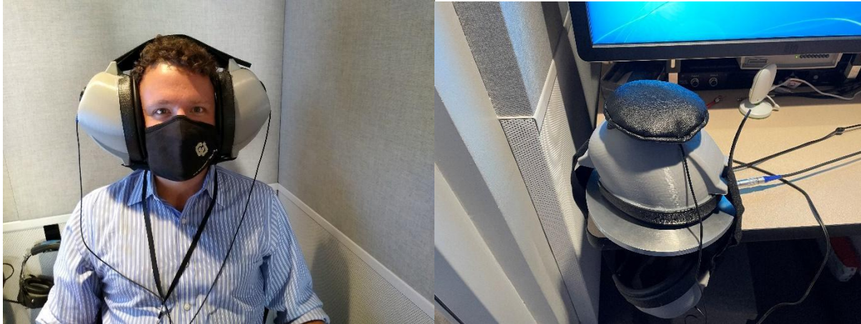
Figure 9. Left: Custom extra-large-volume earphones on the custom flat plate adapter during calibration. Right: Demonstration of use of the earphones; adjustable straps are used to position and secure the earphones over earmuff-style HPDs.
