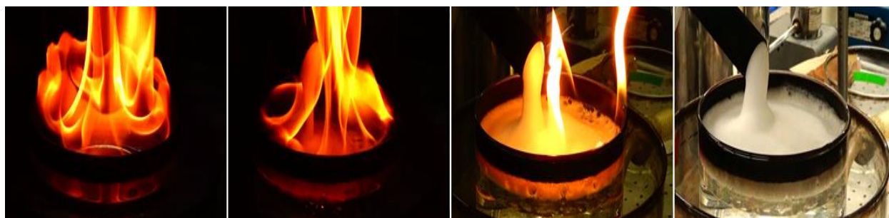
Figure 43. A pool (12-cm diameter, n-heptane liquid, 2-cm lip) fire extinction by foam applied at the center at a constant flow rate; from 30-sec pre-burn to extinction.
