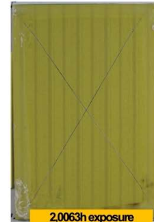
Good corrosion resistance
