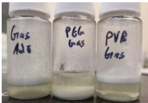
Figure 27. Uncoated A20, PEG, and PVB microspheres with gasoline.
