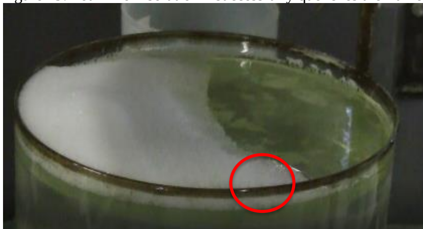
Figure 20. As indicated inside the red circle, as the foam from solution 2 dissipates, the microspheres can be seen floating between the gasoline and water layers
