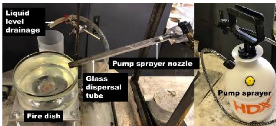
Figure 23. Photographs of new HGM foam sprayer setup
