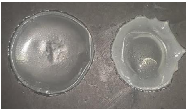
Figure 3. The film with a lower amount of siloxane (left). The film with a higher amount of siloxane (right)
