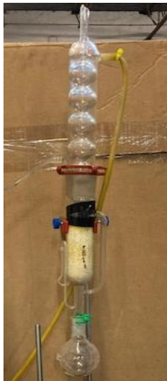
Figure 8. Alcohol extraction of organic chemicals from banana peel powder.
