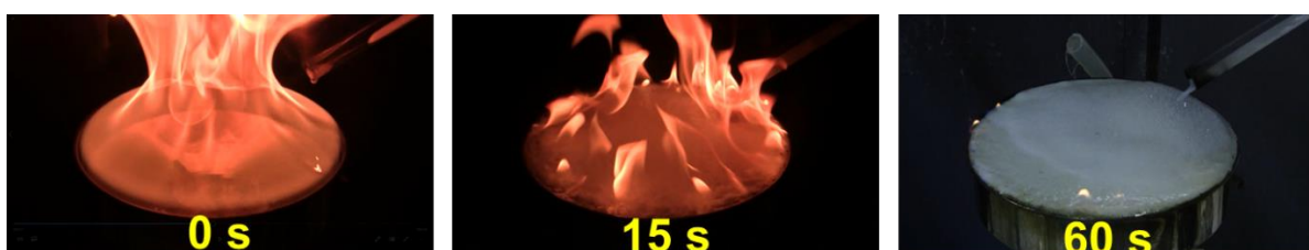
Figure 13. Time lapse image of benchtop fire testing of banana cellulose foam formulations
