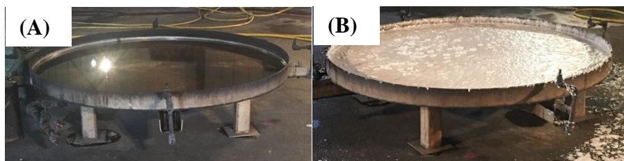
Figure 5. 6 ft diameter pool fire pan with (A) Fuel and (B) Foam on top of fuel after the extinction of fire
