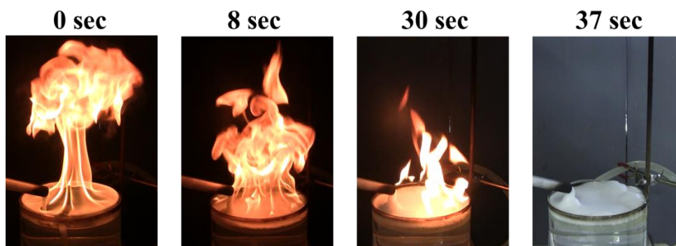
Figure 9. Time-lapse images of gasoline pool fire testing with 1.5% poly(trisiloxane) + 0.8% bmim-DDBS ionic liquid
