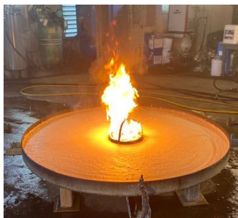
Figure 5. Photograph of 28 ft 2 pool fire testing pan with burnback fire in the middle
