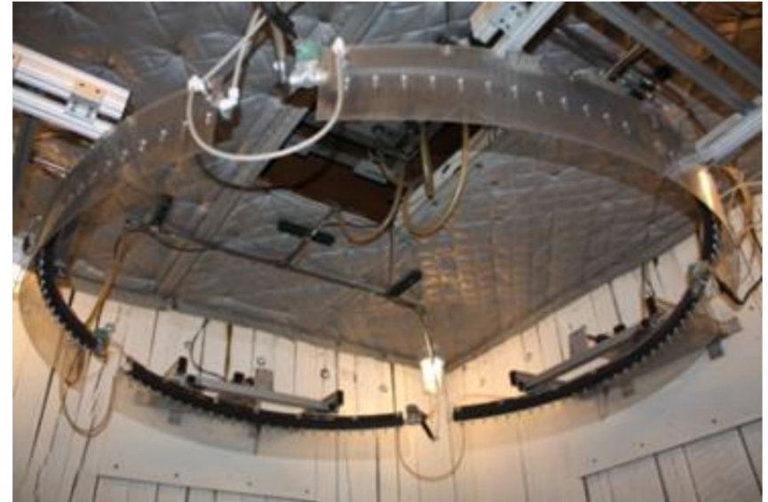
Figure 2: Curved Manifold Quadrants to Simulate Rainfall
