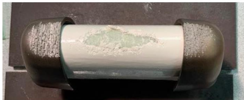
Figure 4: Specimen ID 1-2 after Rain Exposure at 440 MPH
