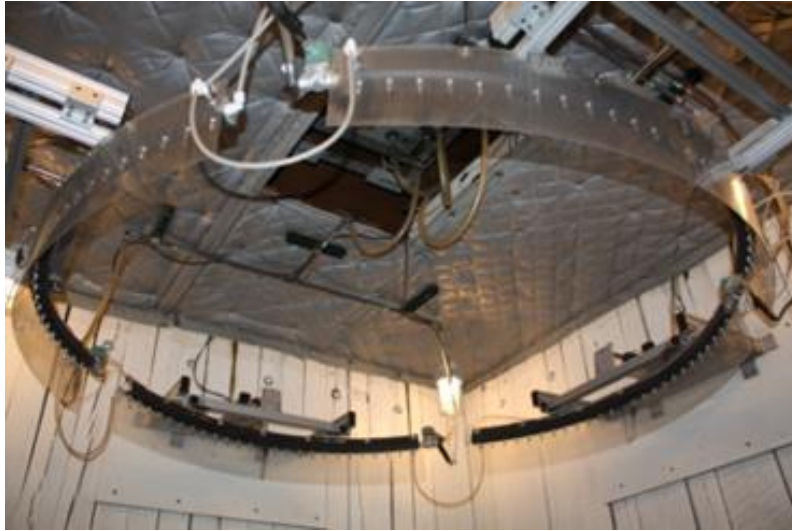
Figure 2: Curved Manifold Quadrants to Simulate Rainfall
