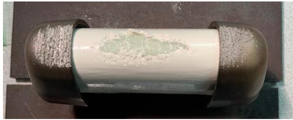
Figure 4: Specimen ID 1-2 after Rain Exposure at 440 MPH
