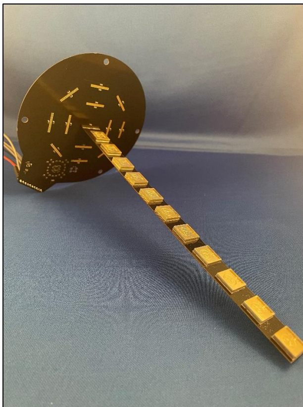
Figure 78: MSND strip inserted into backplate for functionality testing prior to soldering in place.
