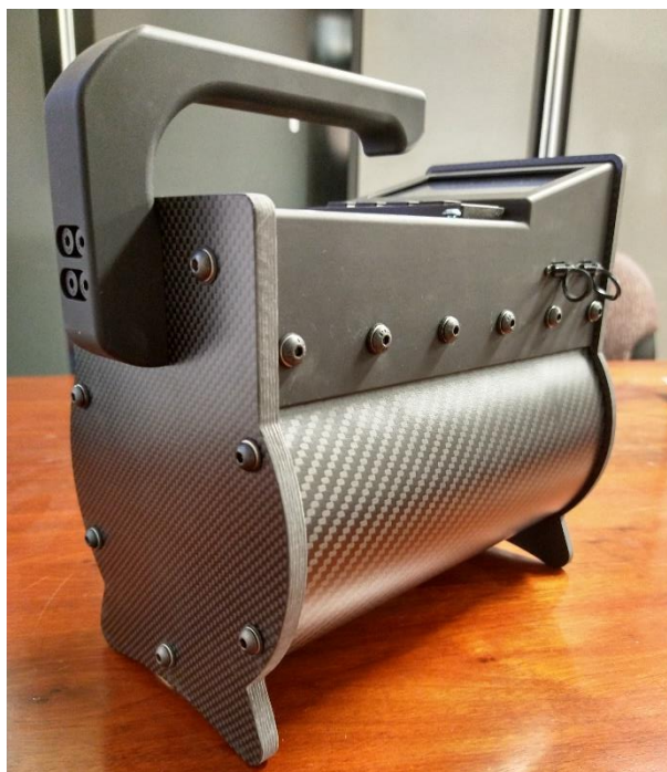
Figure 72: NRID V1 carbon fiber - aluminum case. USB-C ports are used for battery charging (optional, can be swapped) and data I/O.
