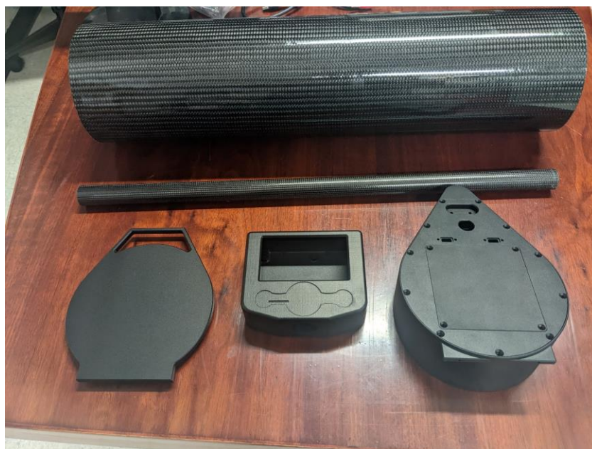
Figure 91: NRID V2 gen. 2 case components. Carbon fiber pieces were cut to size.
