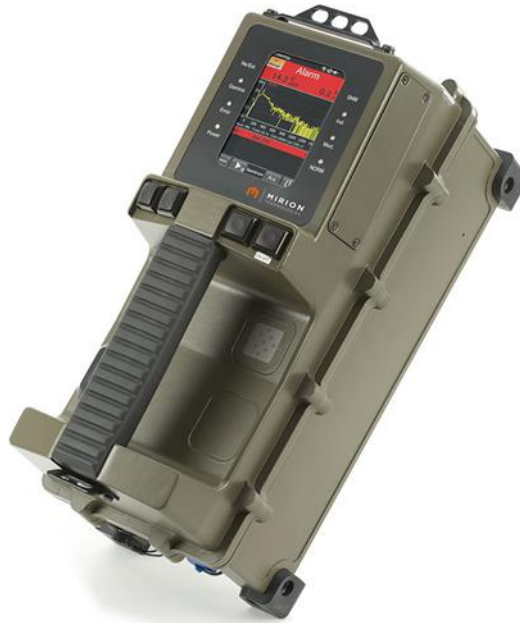
Figure 58: Picture of the Mirion SpiR-ID gamma-ray ID instrument ruggedized for military use. The NRID were packaged in a similar designed handheld housing.
