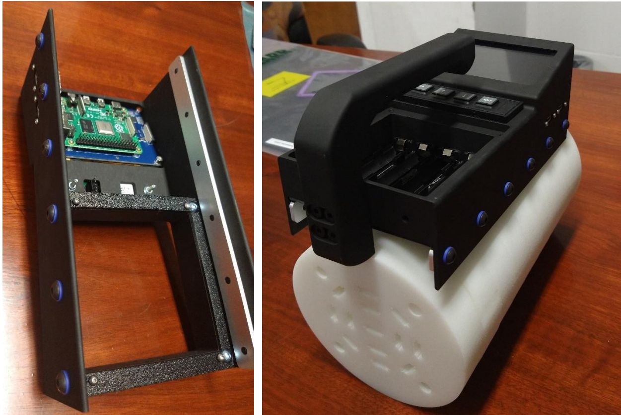
Figure 65: Anodized aluminum components of the NRID V1 gen. 1 case have been machined and assembled.
