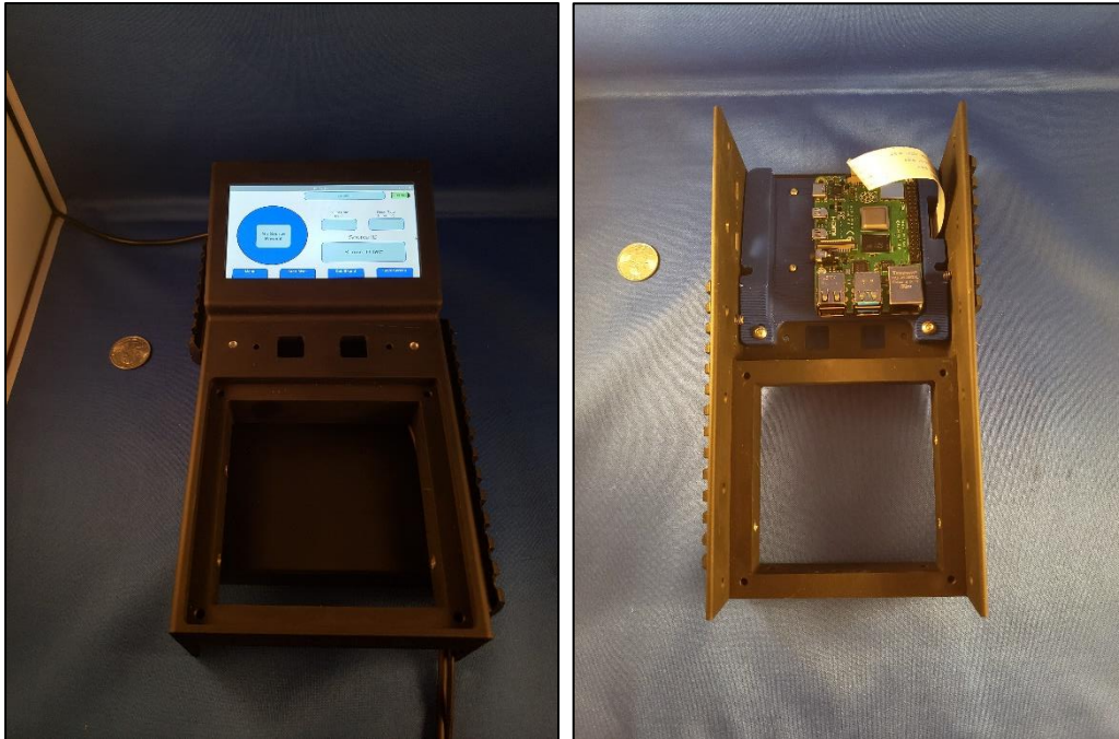
Figure 71: Updated NRID V1 top plate with rails for sling mounts and the screen and Pi-computer bracket.
