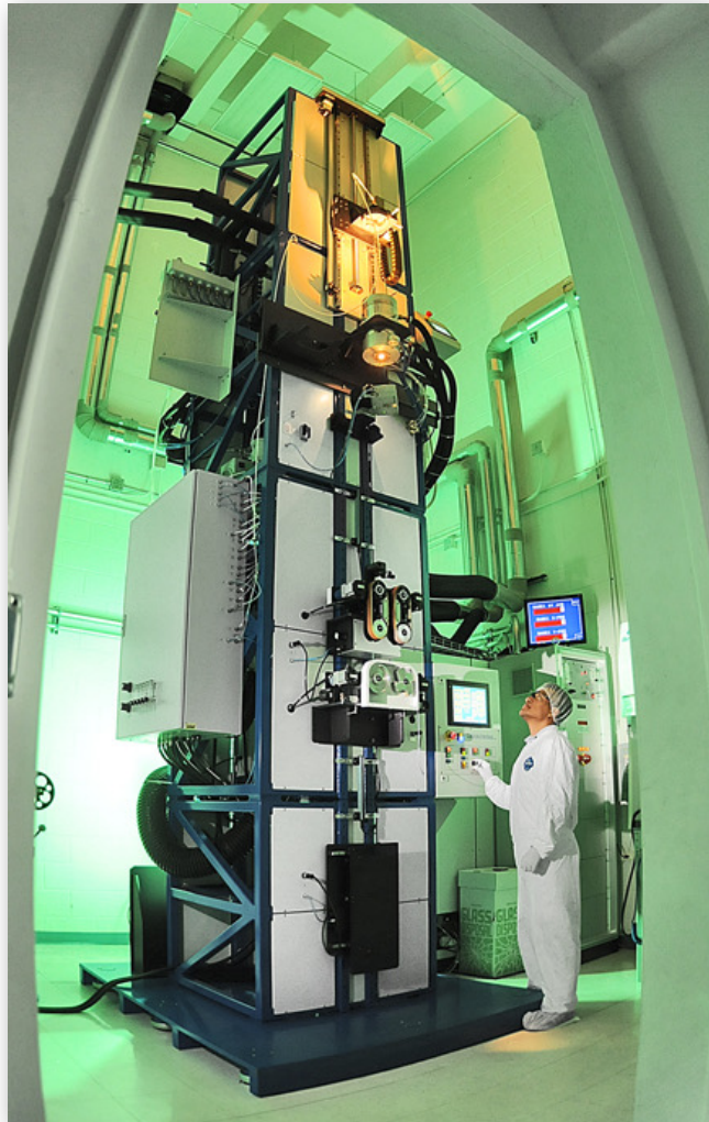
Draw Tower for Microstructured Optical Fiber Fabrication
