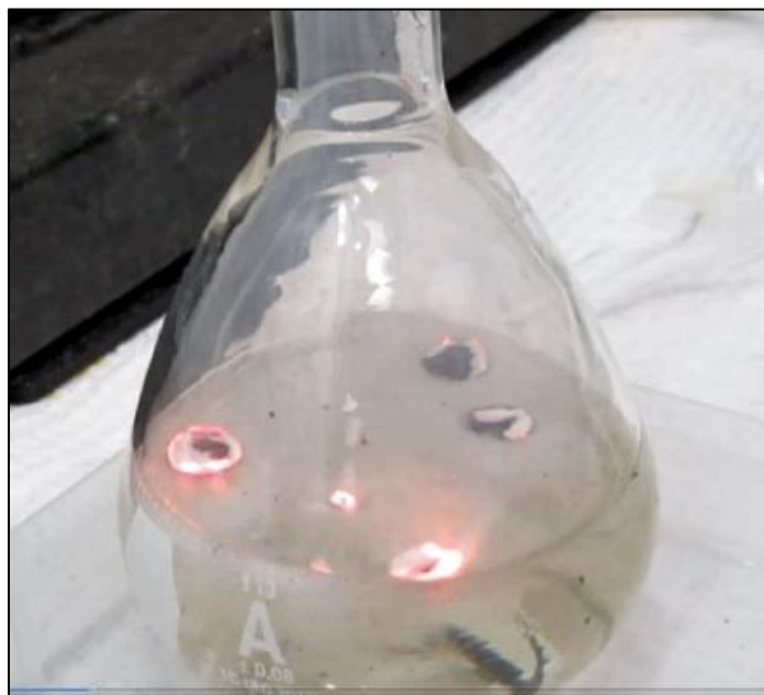
Figure 8. Pellets of \text{Li}_3\text{N} floating in water. Pellets can become red hot when they are not submerged in liquid.
