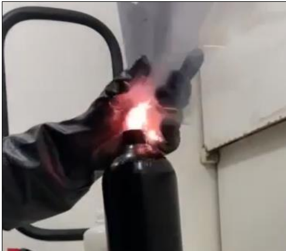
Figure 1. Addition of \text{Li}_3\text{N} pellets to a 1 L DMMP reaction in an open pressure vessel. Reaction of \text{Li}_3\text{N} with water generated a spark that ignited the DMMP vapor. The image is a still frame from a video recording.
