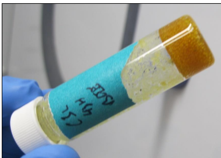
Figure 14. Gelled BCEE– \text{Li}_3\text{N} –pyridine–MeOH reaction after reacting overnight. Typical \text{LiOH} reaction products (gray and white powder) did not form.
