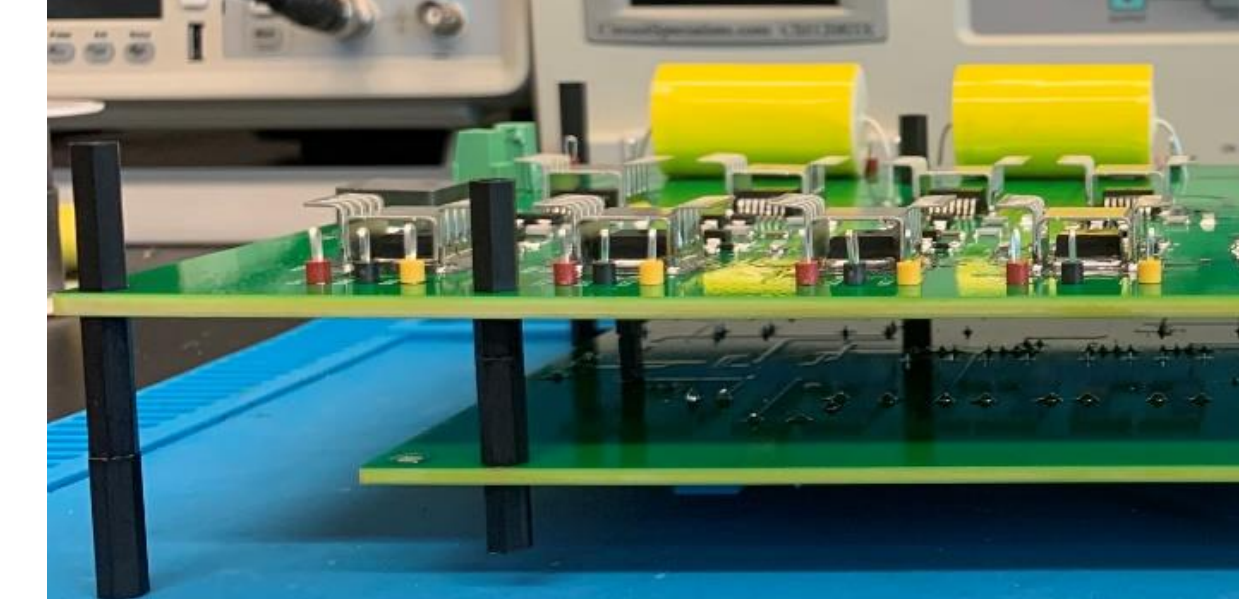
Prototype of a modular 10 kV rated negative DC power supply
