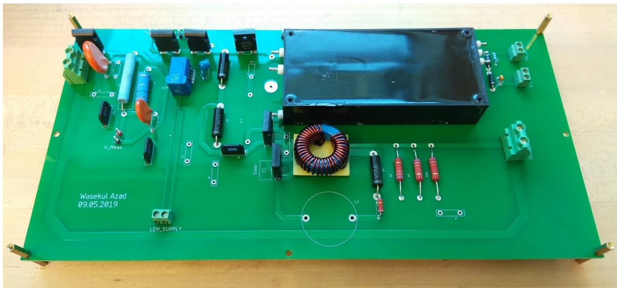
Figure A1. In-house prototype of HV power conditioning circuit for pulse forming network.
