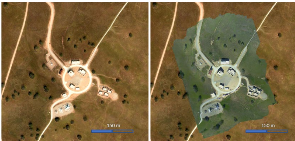
Figure 22. VRICON Data over Camp Roberts (left). Merged VRICON and Puma FMV data after registration (right).
