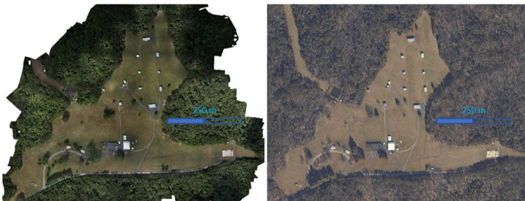
Figure 8. Freya drone (left) and BuckEye (right) orthomosaic outputs (right).
