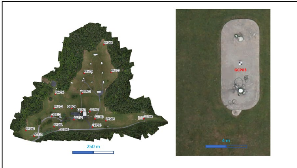
Figure 10. Checkpoints used to assess co-registration accuracy between the Freya and BuckEye reference data. The spatial distribution is shown on the left side, while a detail of a painted target is shown on the right.
