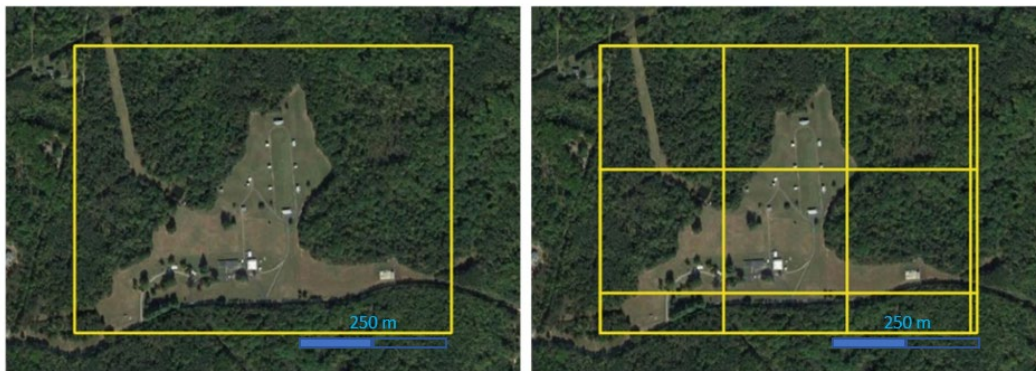
Figure 11. Depiction of Quick versus Tiled processing approaches. The left side shows the Quick approach for the Corbin data set. The yellow box has been resampled into a single tile with 3,000 pixels in the long (horizontal) direction. The right side shows the Tiled approach, the larger boxes are 3,000 × 3,000 pixels, while smaller, “remainder” boxes are shown on the bottom and right edge.
