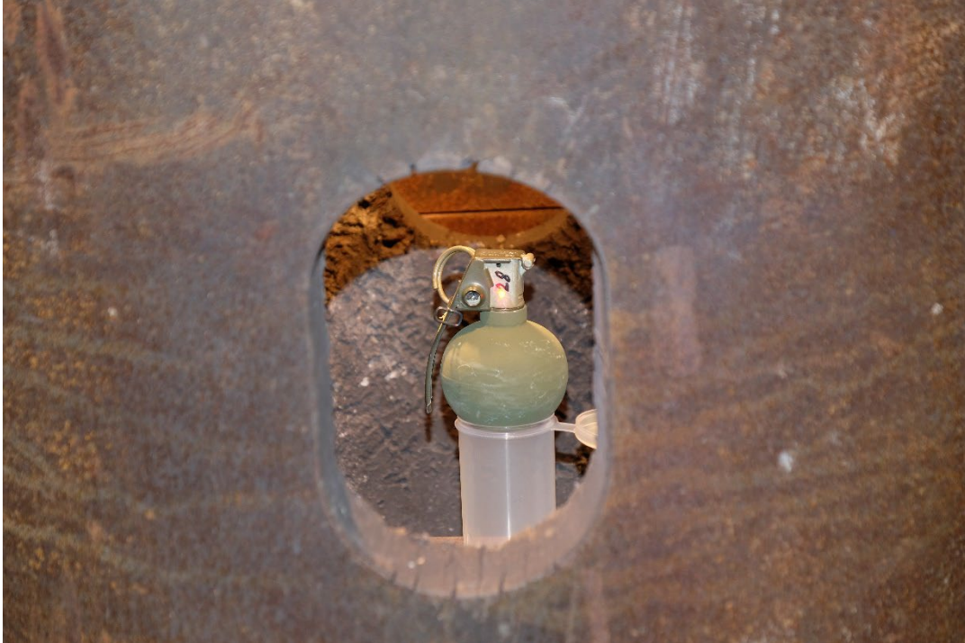
Figure 2 View along the shot line on a M67 hand grenade inside a firing pot
