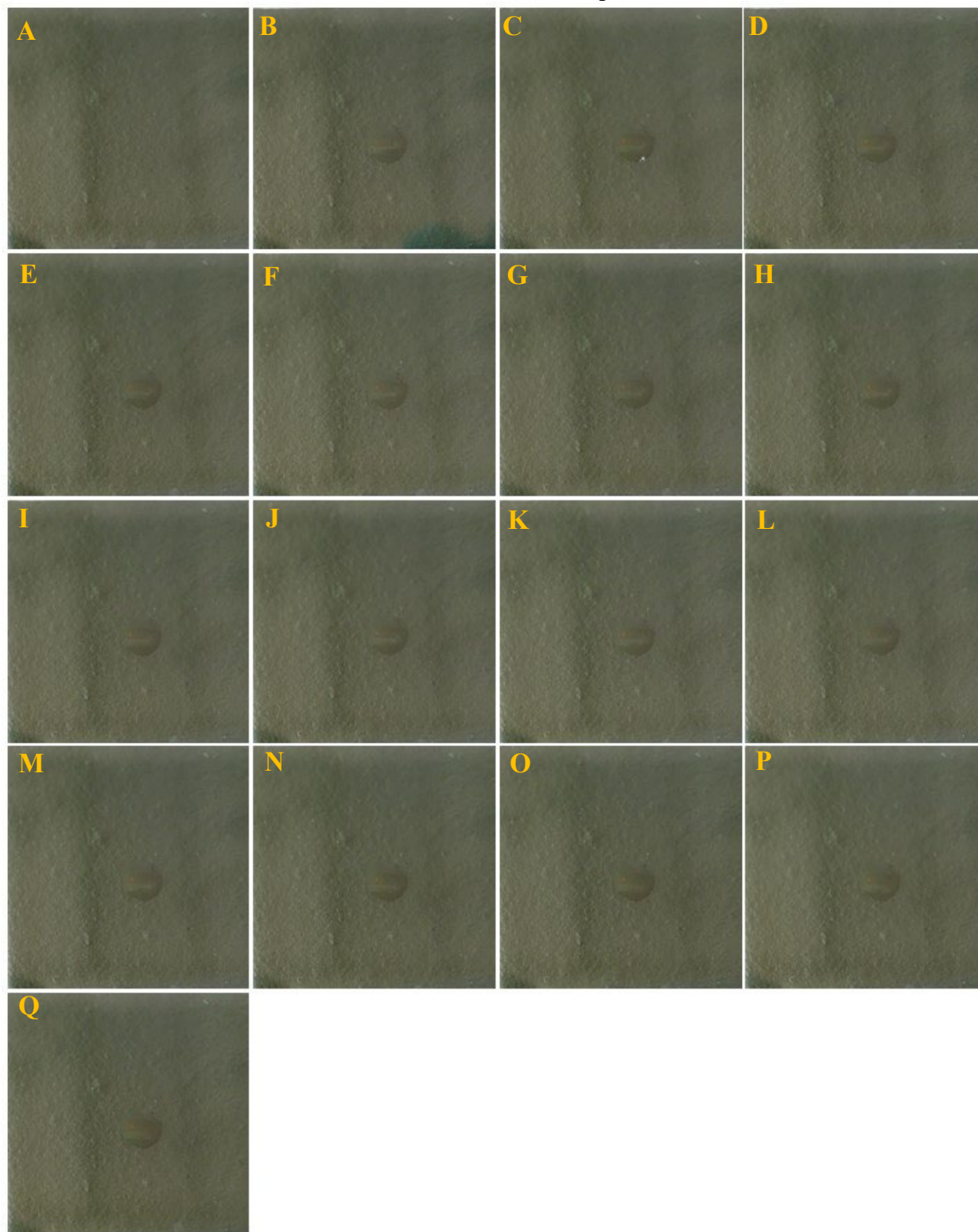
Fig. B1 — DFP on 11 wt% coated. Images of a film supported by painted coupon before application (A) and at 0 (B), 0.5 (C), 1.0 (D), 1.5 (E), 2.0 (F), 2.5 (G), 3.0 (H), 3.5 (I), 4.0 (J), 4.5 (K), 5 (L), 10 (M), 15 (N), 20 (O), 25 (P), and 30 (Q) min following application of the target. These images were collected with a glass cover in place to limit evaporation. Reflections from the cover can be seen in some images.
