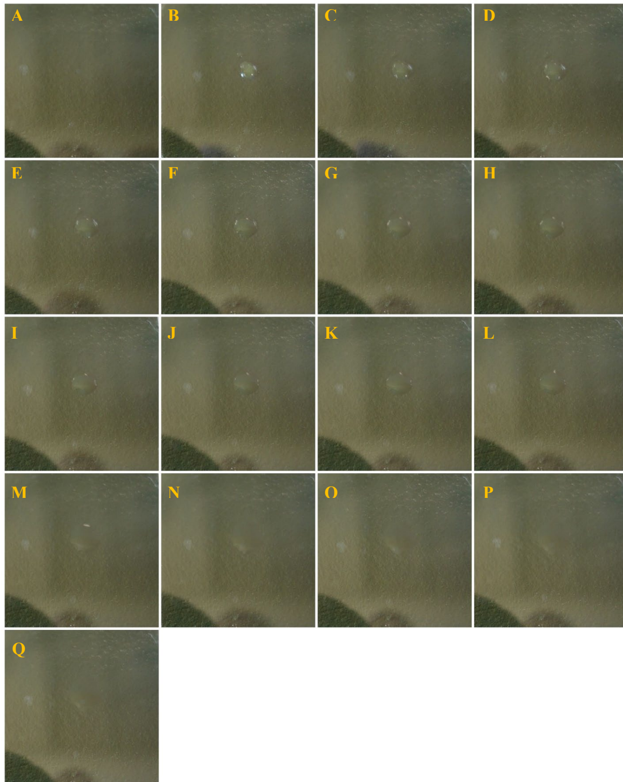
Fig. N1 — DFP on PFTS extra high ECA spray coated. Images of a coupon before application (A) and at 0 (B), 0.5 (C), 1.0 (D), 1.5 (E), 2.0 (F), 2.5 (G), 3.0 (H), 3.5 (I), 4.0 (J), 4.5 (K), 5 (L), 10 (M), 15 (N), 20 (O), 25 (P), and 30 (Q) min following application of the target. These images were collected with a glass cover in place to limit evaporation. Reflections from the cover can be seen in some images.
