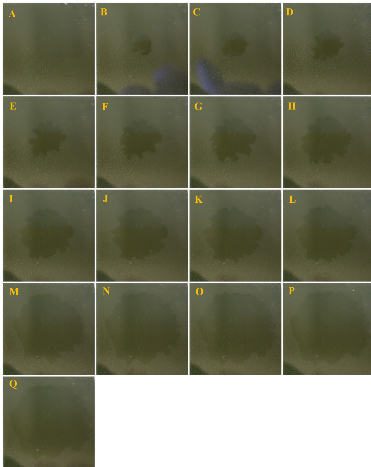
Fig. B1 — DFP on PPGDI. Images of a film supported by painted coupon before application (A) and at 0 (B), 0.5 (C), 1.0 (D), 1.5 (E), 2.0 (F), 2.5 (G), 3.0 (H), 3.5 (I), 4.0 (J), 4.5 (K), 5 (L), 10 (M), 15 (N), 20 (O), 25 (P), and 30 (Q) min following application of the target. These images were collected with a glass cover in place to limit evaporation. Reflections from the cover can be seen in some images.
