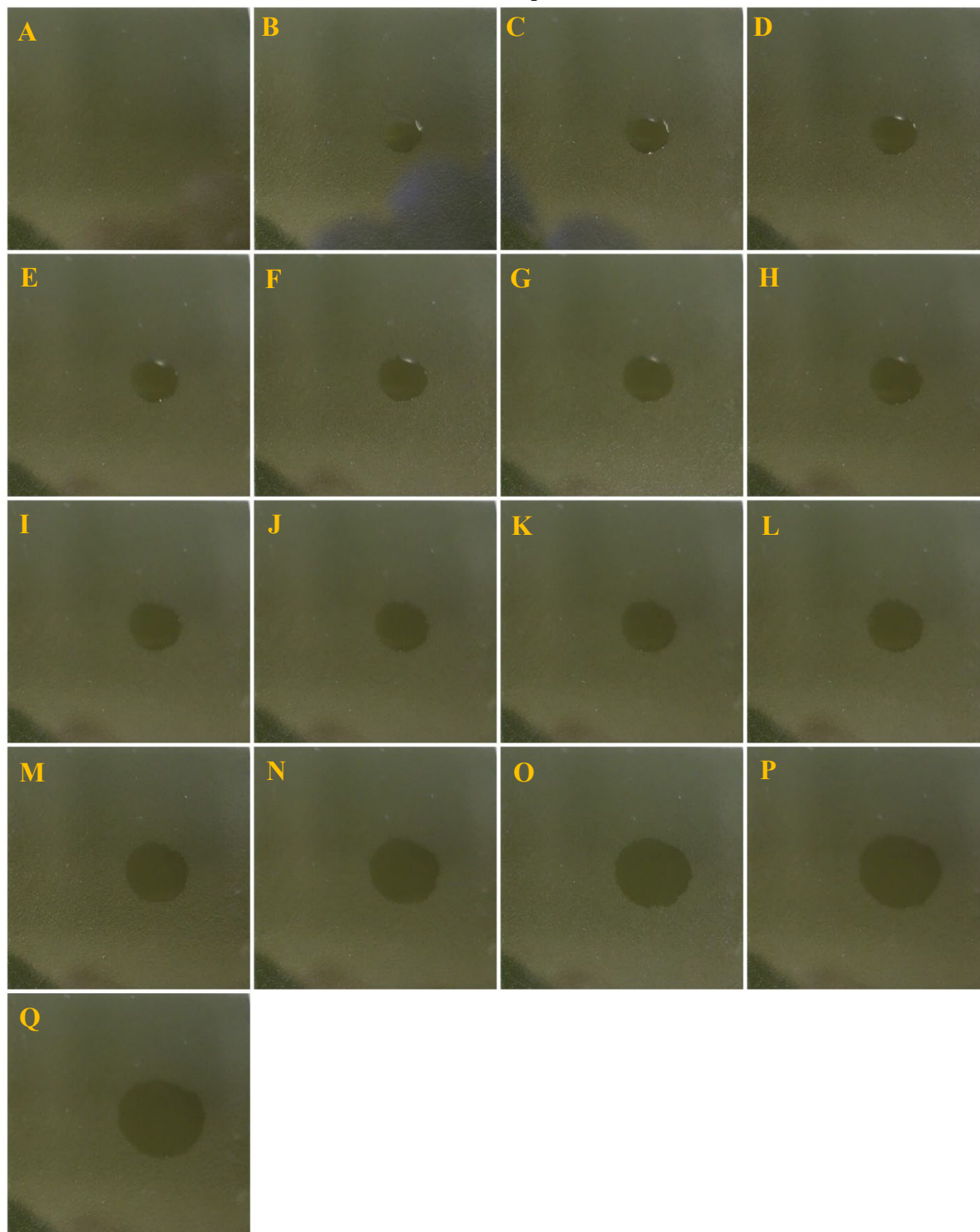
Fig. D1 — DFP on 50:50 PPGDI/PDMS. Images of a coupon before application (A) and at 0 (B), 0.5 (C), 1.0 (D), 1.5 (E), 2.0 (F), 2.5 (G), 3.0 (H), 3.5 (I), 4.0 (J), 4.5 (K), 5 (L), 10 (M), 15 (N), 20 (O), 25 (P), and 30 (Q) min following application of the target. These images were collected with a glass cover in place to limit evaporation. Reflections from the cover can be seen in some images.
