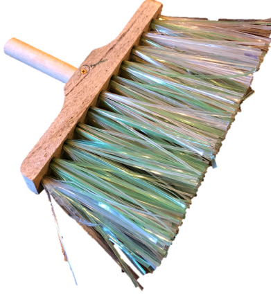
Figure 6: A broom whose bristles are made from 2L plastic bottles.
