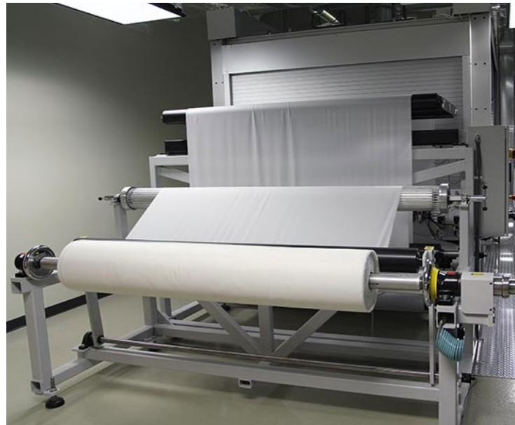
Roll to Roll fabric treatment equipment (LaunchBay LLC)
